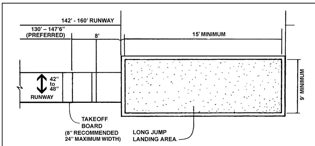
**LONG JUMP AND TRIPLE JUMP** — The declination in the approach shall be limited to 2:100 (2%) laterally and 1:1,000 (0.1%) downward in the jumping direction.
